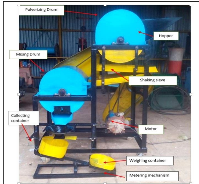
Fig. 4 : Media Mixture Machine for Horticultural Crop Nursery.
